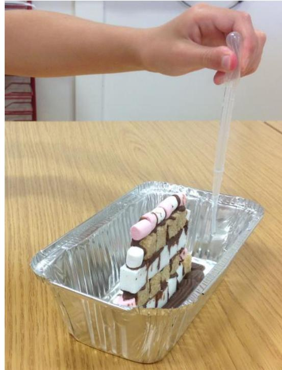
Note: The sugar cubes used in these model walls will dissolve in water, however real stone does not dissolve in water. The salts within the stone will dissolve though and they will move through the stone and cause problems.
